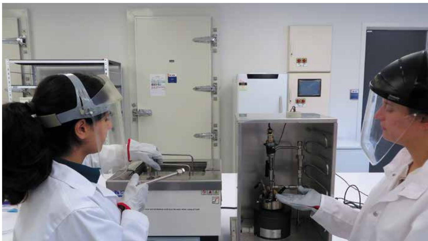
Figure 3. Hydrothermal treatment at lab scale (left) and pilot scale (right)
