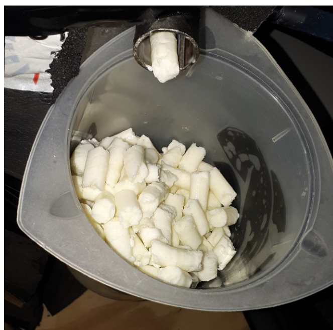
Figure 3: Sheep milk frozen during an initial trial with an early larger-scale tube freezer prototype
