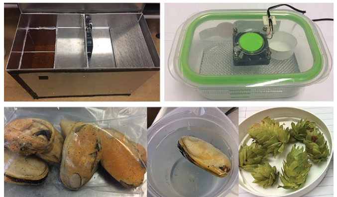
AFD small scale trial units and examples of dried product
