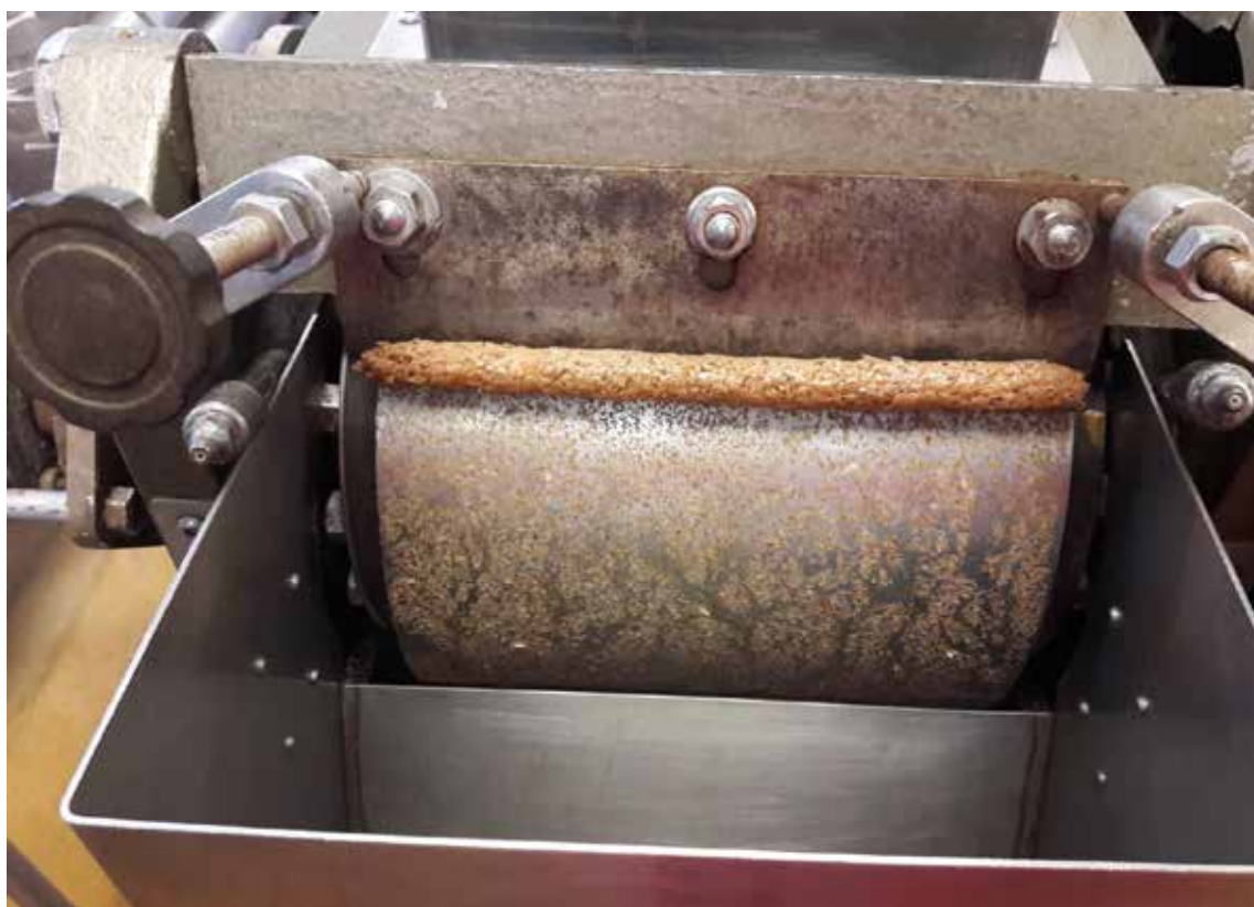
Pilot drying creamed pomace for milling to a powder – one option
